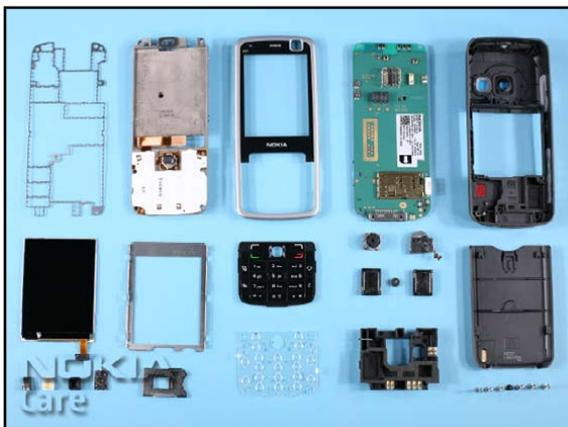
28. The disassembly procedure is now finished.
