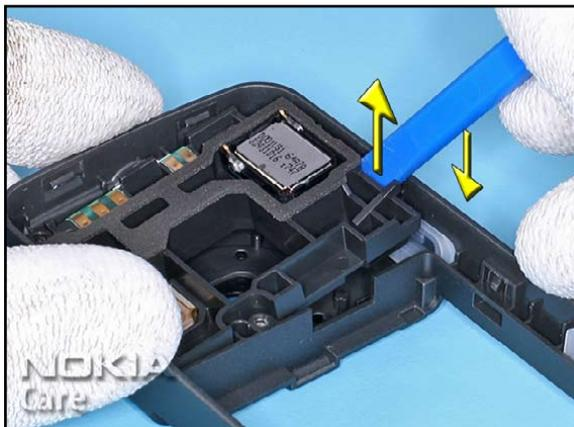
24. Unlock and remove the ANTENNA MODULE ASSEMBLY.
