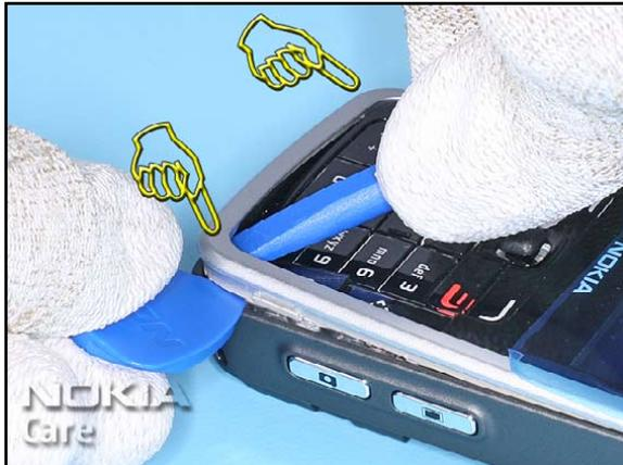
4. Place the SS-93 between the KEYMAT and the edge of the A-COVER and unlock the bottom clip first. Hold the SS-93 in the shown position and unlock the side clip with SRT-6 by pressing it between the A-COVER and the B-COVER. Do the same on the other side.
