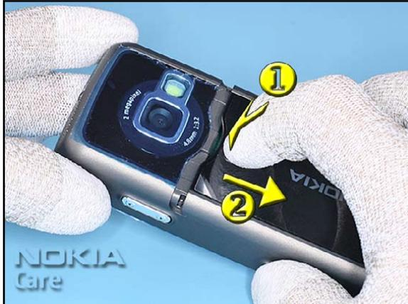
2. Cover all sensitive surfaces with a protective film. Unlock and open the C-COVER ASSEMBLY. Remove the Battery if inserted.
