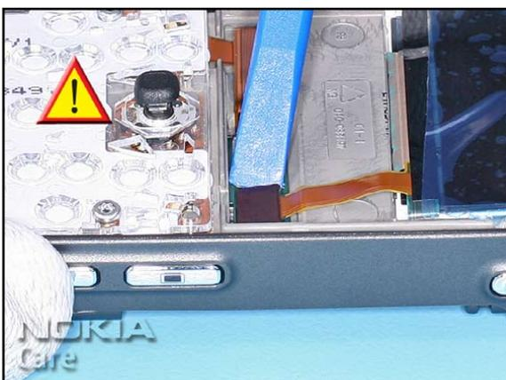
10. ...and disconnect it from the ENGINE MODULE.
