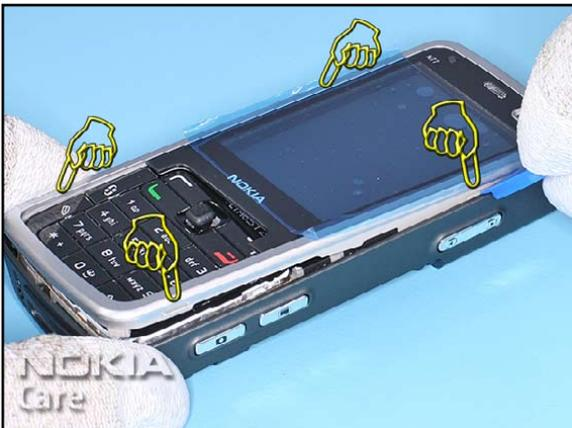
5. Slide the SRT-6 along the marked edges to unlock the snaps.
