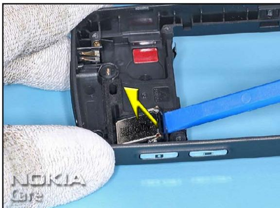
27. Remove the IHF SPEAKER from the B-COVER. The DC-Jack and the MICROPHONE can be removed easily.
